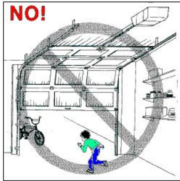
To check the garage door, the garage door opener must be detached from the door while in the closed position. On most openers manufactured since 1982, a "quick-release" mechanism is provided which permits the opener to be detached from the door.
